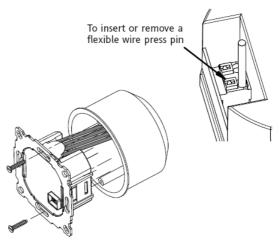
The plastic tab must be in place to provide insulation between the terminals/wires and the mounting screw.
